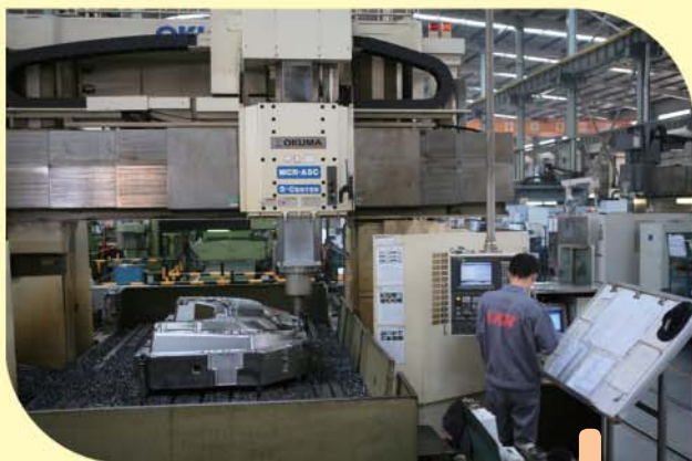
Production of mould base for the instrument panel of an automobile needs stock of big steel block together with proper heavy-duty machines 生產汽車儀表板的模架需要大型鋼塊存倉及配合適合的重切削機床
