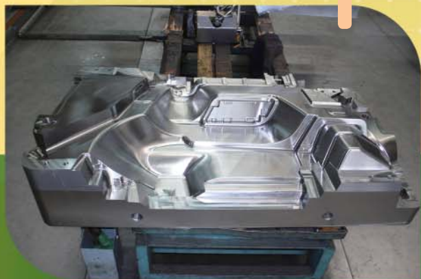
Using high speed and efficient machines to shorten the production time and enhance the surface finishing of mould base 使用高速及高效能切削機床可以縮短生產時間及提升模架表面光潔度
