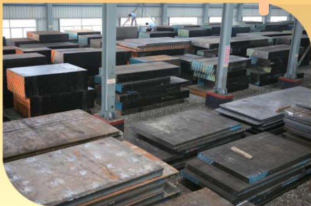
Forging blocks and hot roll plates are the basic materials for large size mould base 大型鍛件及熱軋鋼塊乃大型模架的主要原材料
