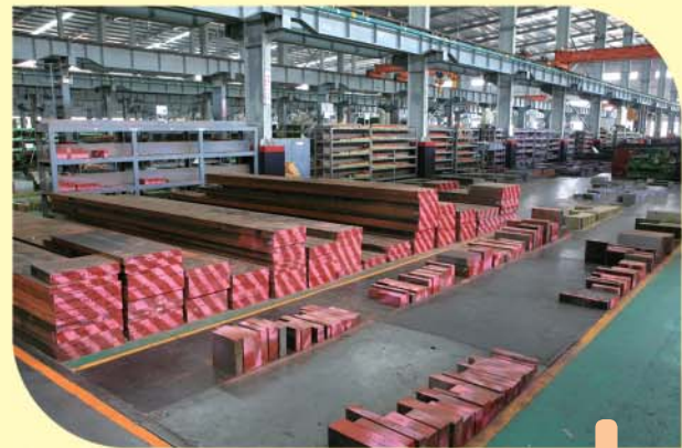
Using the colour code to distinguish different steel types systematically 使用顏色代碼有系統地分辨各種鋼材
