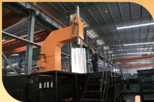
Using the vertical band saw to cut away the residual material in order to save time and cost in the milling process 使用大型立式帶鋸將餘料切走可省卻用於銑床的時間及成本
