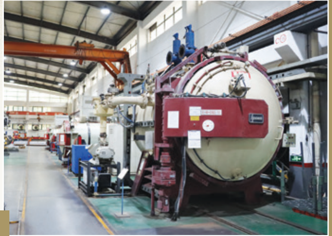
真空熱處理爐提供穩定的熱處理加工服務 Vacuum furnaces provide stable heat treatment services
