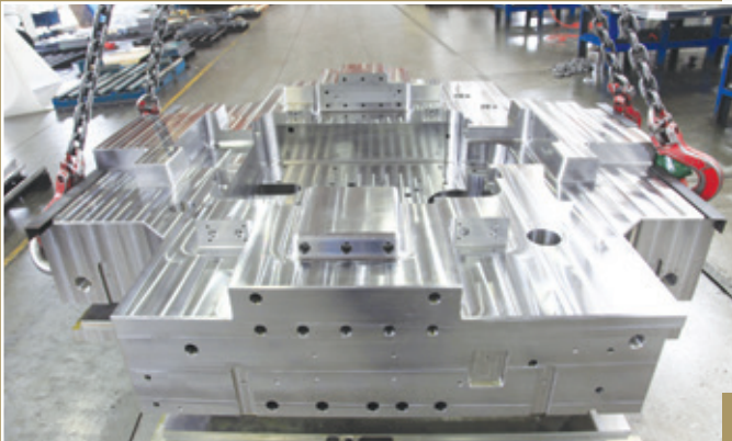
大型非標模架部分 Part of a large size custom-made mould base
