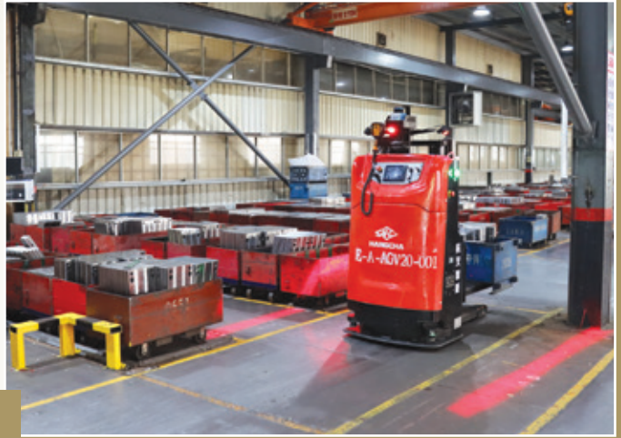
無人駕駛電動搬運車正在搬運模板 The driverless electric truck is moving the mould plates
