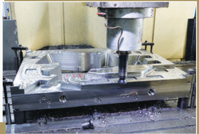
一件大型非標模架正進行加工 A large size custom-made mould base is undergone machining
