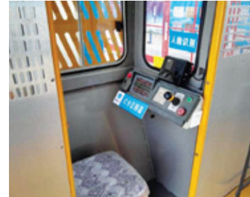
Driver of construction elevator face recognition system
