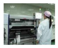
• Fix surface mount device (SMD) components onto PCB by SMT machines
