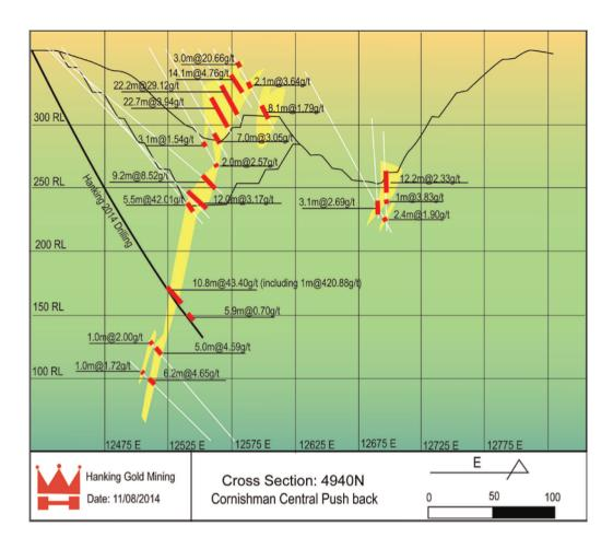
Figure 1 - Profile of 4940N exploratory line of the Cornishman Gold Mine
